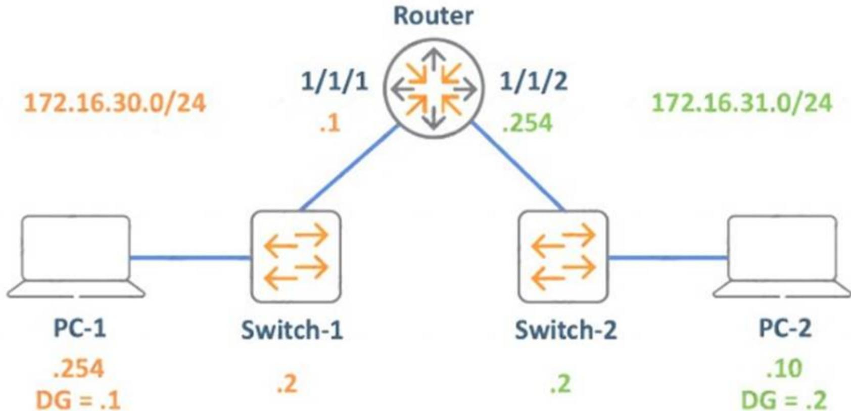
The PCs are not able to successfully establish bidirectional communication. What change must you deploy to enable the communication between PC-1 and PC-2?
