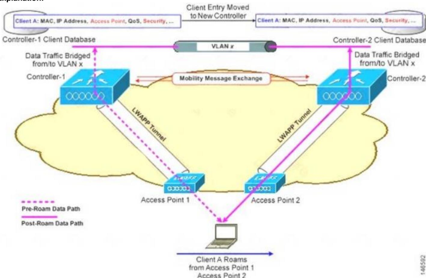
In this instance controllers exchange mobility control messages (over UDP port 16666) and the client database entry is **moved** from the original controller to the new controller.
